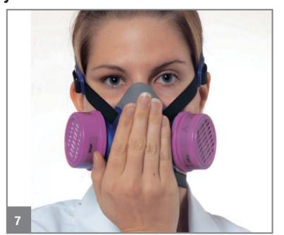
Positve pressure test: Seal the exhalation valve of half mask and exhale. The half mask will inflate slightly. If the exhaled air leaks out of the mask, readjust the face piece and adjust the straps or use a different mask size. Repeat test until a successful seal check is met.
