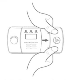
(2) If replacing batteries, remove the old batteries and properly dispose of them as recommended by the battery manufacturer. If installing 2 new AA batteries, note the polarity illustration in the battery compartment. When batteries are correctly installed, the alarm horn sounds one beep.
